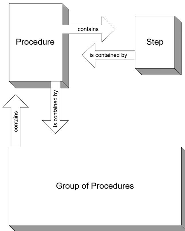
The class defines its components in a certain sequence within a single hierarchy. The standard tells us how many components are allowed or required, in what order, and which ones are just optional. The relationships between objects are defined in a content model, known in XML as a Document Type Definition, or schema.
